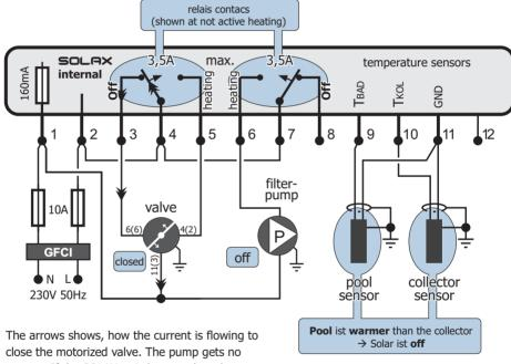
current. If the SOLAX switches on, the relay
