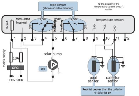
In this example, the collector sensor is warmer than the bath sensor  $\rightarrow$  the SOLAX switches on. The arrows shows, how the current flows over the filter pump and solar pump.
